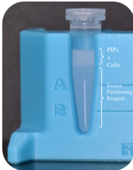
Figure 3. Emulsified PIPs and cells are seen in the top phase while the excess waste Partitioning Reagent is in the bottom phase.
