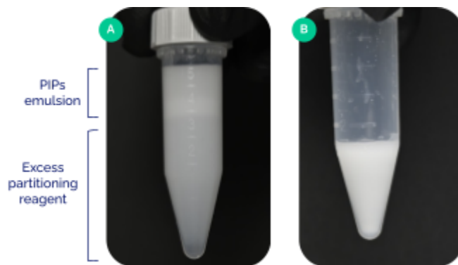
Figure 5. PIP tubes after removing them from the Dry Bath (A) and after discarding the remaining excess Partitioning Reagent and CLB3 emulsion (B).
