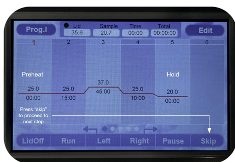
Figure 1. Dry Bath interface programmed for cell lysis protocol. Both “preheat” and “hold” functions are depicted as “00:00” on the Dry Bath interface. In order to start pre-heating, one must first press “run”. When samples are inserted, press the “Skip” and then “yes” to continue the protocol.
