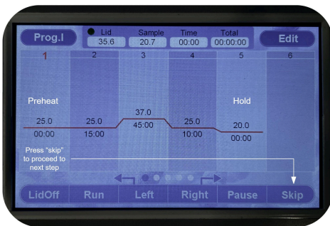
Figure 1. Dry Bath interface programmed for cell lysis protocol. Both “preheat” and “hold” functions are depicted as “00:00” on the Dry Bath interface. In order to start pre-heating, one must first press “lid on” and “run”. When samples are inserted, press the “Skip” and then “yes” to continue the protocol.
