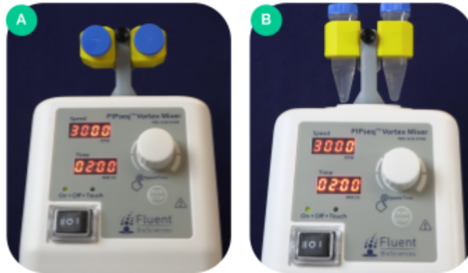
Figure 2. The rotating vortex adapter shown in the horizontal configuration (A) and the vertical configuration (B).
