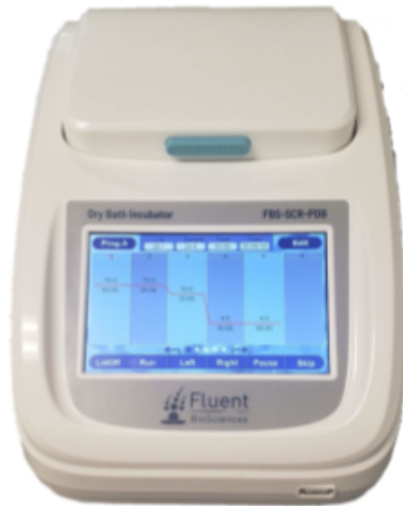
Figure 5. The PIPseq™ Dry bath to be used for the lysis incubation step.
